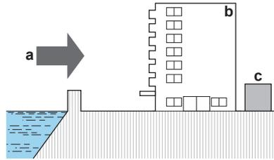
If the outdoor unit is exposed to direct sea winds, install a windbreaker.
