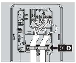
Tighten the terminal screws securely. We recommend using a Phillips screwdriver.
