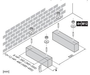
a Make sure not to cover the drain holes of the bottom plate of the unit.
