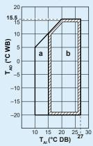
${\bf a}$ : Warming up operation range;  ${\bf b}$ : Heating operation range;  ${\bf T}_{\rm Al}$ : Ambient indoor temperature;  ${\bf T}_{\rm AO}$ : Ambient outdoor temperature
