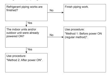
It is very important that all refrigerant piping work is done before the units (outdoor or indoor) are powered on. When the units are powered on, the expansion valves will initialise. This means that the valves will close.
