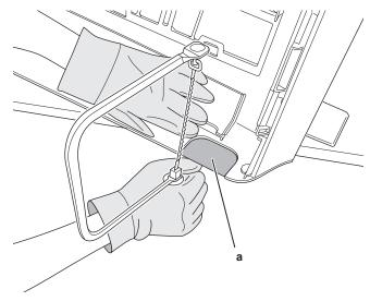
2 Remove any burrs along the cut section using a half round needle file.
