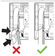
2 Pass the drain hose and refrigerant piping through the wall hole and seal the gap with a putty.
