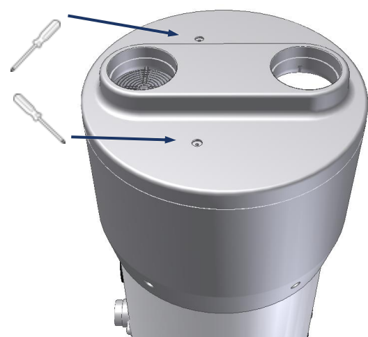
Fig. 18 – Removal of upper cover
